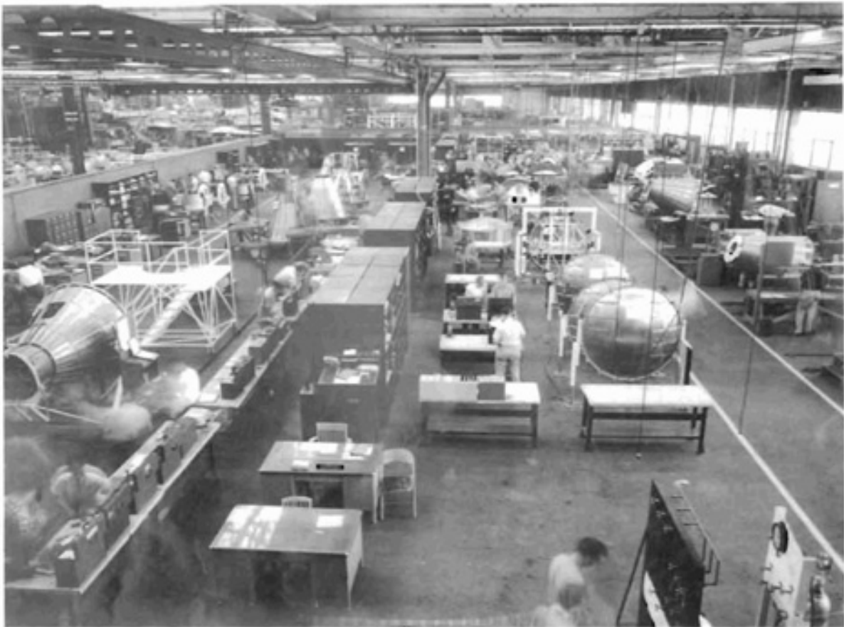
Figure 2 McDonnell's main work area for fabrication of the major components of the Mercury capsules. Source: Box 75, Project Mercury Photographs, Entry No. 70, History Office Source Files, RG 255, NARA-Southwest. (NASA)
