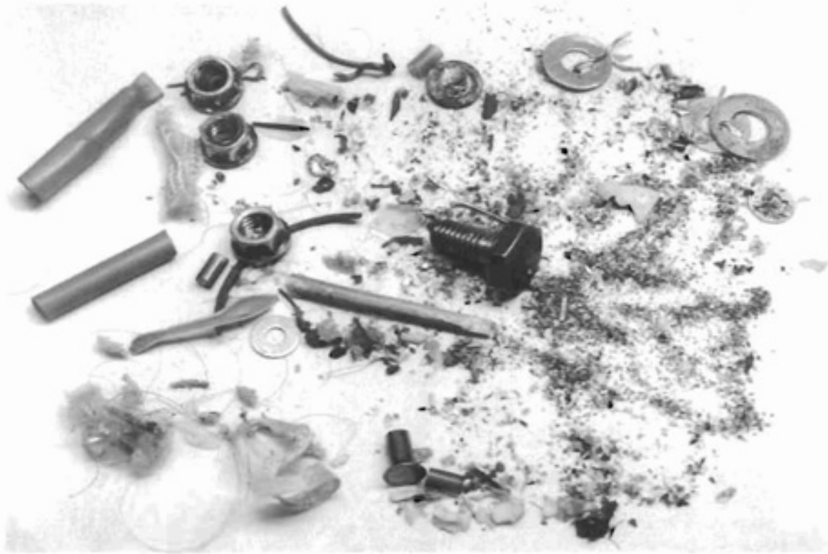
Figure 5 Yield of loose materials from tumbling Capsule No. 13 in December 1961. Source: Box 76, MSC Capsule No. 13 Photos, Entry No. 70, History Office Source Files, Folder 1, RG 255, NARA-Southwest. (NASA)
