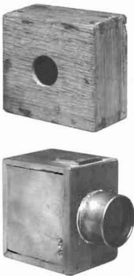
Figure 1 Two examples of Talbot's 'mousetrap' cameras, c. 1835. (Science & Society Picture Library)
