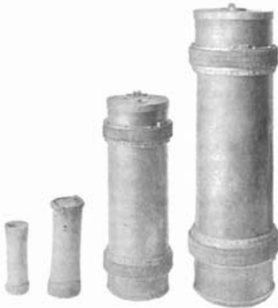
Figure 1 Comparison of carrier sizes, 1898. On the extreme left is a telegram carrier used in Berlin, and next to it is a 3-in telegram carrier from the London system. To its right is a carrier used on the pioneer Philadelphia 6-in mail tube and on the extreme right is the standard 8-in carrier used for all later mail-tube systems. (Published in Transactions of the American Society of Mechanical Engineers in 1899)
